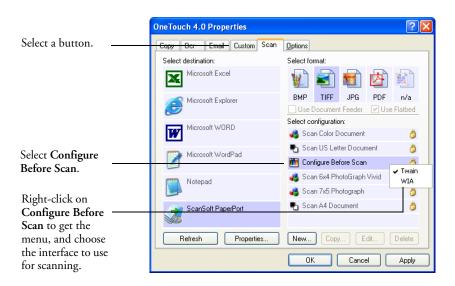
4. Right-click on **Configure Before Scan** and choose an interface to use for configuring before scanning.
