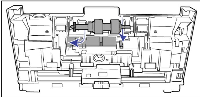
10. Lift the roller cover and carefully push it closed to lock it in place. Make sure everything is aligned properly and the cover is fully closed. If the cover is not fully closed it will break during scanning and damage the scanner.
