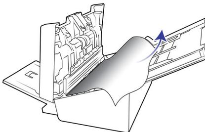
To reduce the number of paper jams, smooth and straighten the paper before scanning, adjust the guides to the paper size, and insert the paper evenly into the ADF.
