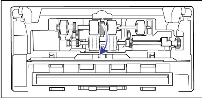
11. Lift the roller cover and carefully push it closed to lock it in place. Make sure everything is aligned properly and the cover is fully closed. If the cover is not fully closed it will break during scanning and damage the scanner.
