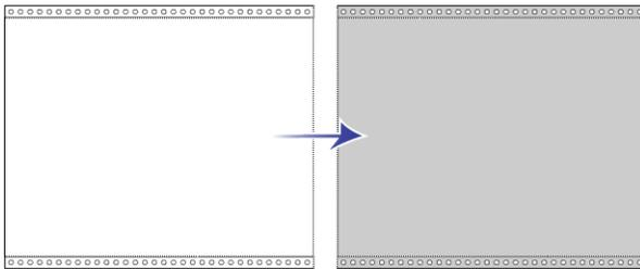
Do not place a stack of connected paper in the input tray. The paper will tear when the separation roller attempts to separate the current page from the rest of the stack. If you want to scan a long document of dot matrix paper, try placing the document stack on the desk behind the input tray. Close the input tray extension and place the leading page in the input tray.
