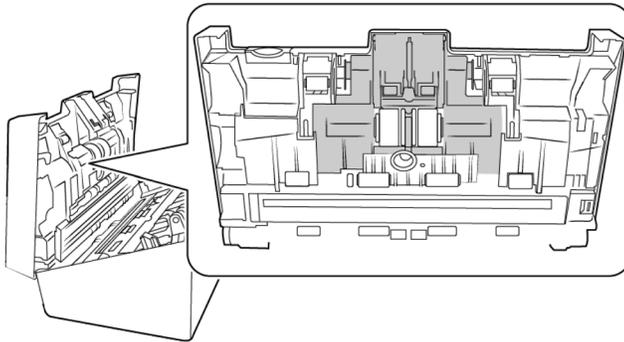
3. Pinch the sides of the roller cover and pull it down to access the roller.
