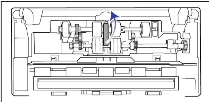
5. The lower roller is held in place with a lock tab that rotates to lock and unlock it. To unlock the tab, rotate it until the small lock flange is completely free.
