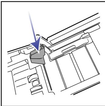
3. You can close the scanner when both paper guides are properly seated in the scanner.
