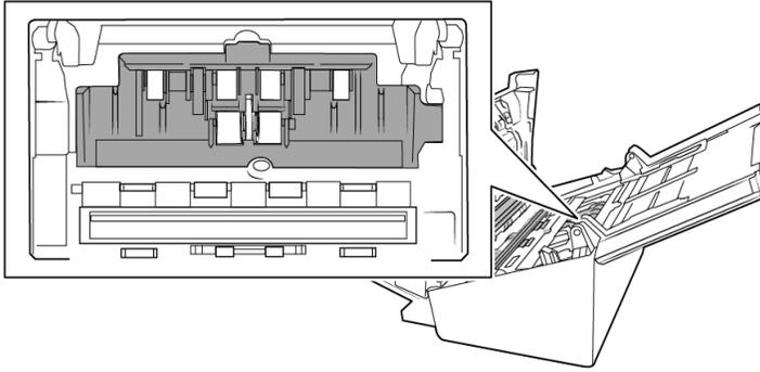
3. Move the paper guides to the side and then pull the feed roller cover away from the scanner.
