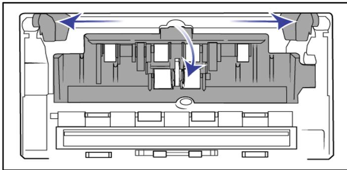
4. Rotate the belt upwards.
