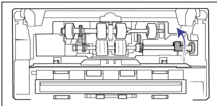
10. Rotate the belt back down into place. The cover will not close if the belt is in the wrong position.
