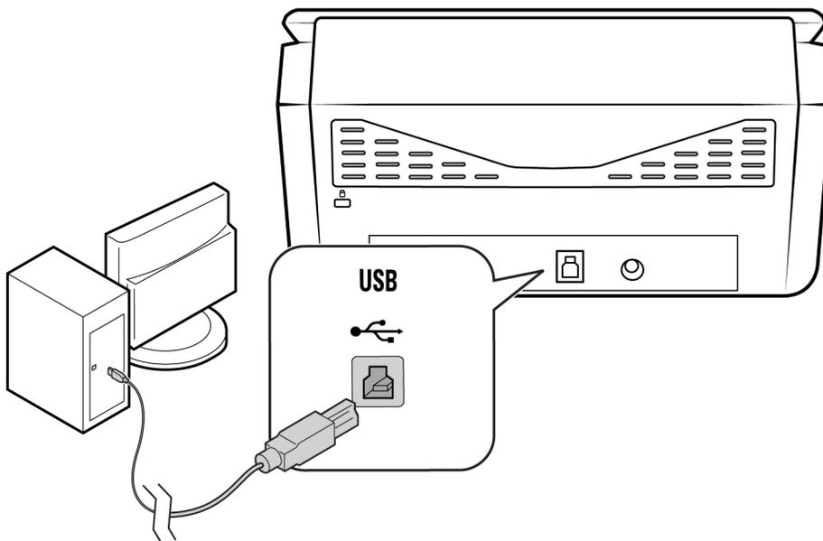
**Note:** Only use the USB power cable included with your scanner. Connecting any other type of USB power cable may damage your scanner, and will void its warranty. If you do not have your USB power cable, you can order a new one by contacting our Customer Service department. Please refer to the Technical Support Card, included with your scanner, for our company contact information, or visit the Parts & Accessories page for your scanner at [www.visioneer.com](http://www.visioneer.com).
