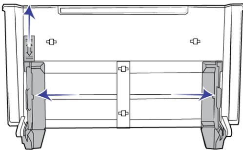
3. Flip up the paper guides, extend the input and output trays.
