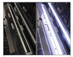
Light Bar – An advanced light array increases the amount of light sources from 1 LED to 45 LEDs, providing superior lighting to produce superior images. Ultrasonic Multi-Feed Detection allows you to correct overlapped paper by detecting paper thickness between documents. If two documents are detected, the user will be alerted to make corrections before the scanning resumes, ensuring every page is captured.
