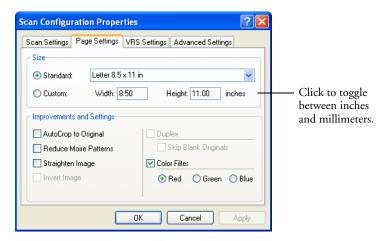
**Size**—Click **Standard**, click the menu arrow and choose a page size from the list, or click **Custom** and enter the horizontal and vertical page dimensions in the boxes. The maximum size is 8.5" by 14". The units of measurement can be inches or millimeters. Click the name of the units, inches or millimeters, to toggle between them.
