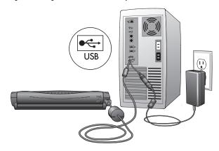
The USB symbol, as seen in the above diagram, identifies the location of the USB port on your computer. If the plug does not attach easily, make sure that you are plugging it in correctly. Do not force the plug into the connection.
