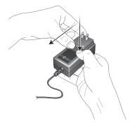
4. To place a new adapter on the power supply, use the procedure described on page 12 of this User's Guide.
