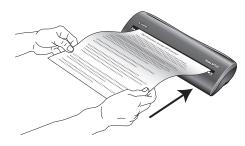
2. The AutoLaunch technology senses that a document is inserted into the page feed and starts the scanning. The scanner rollers will grab the top edge of the paper and begin to scan and feed the document through the scanner.
