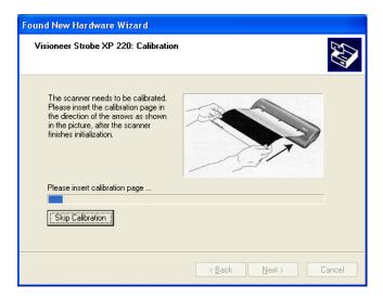
6. Insert the calibration page into the page feed in the direction of the arrows on the page.
