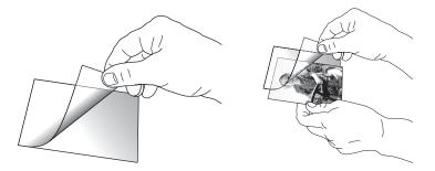
2. Now insert the photo and sleeve into the scanner's page feed with the clear plastic and image facing up.
